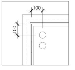
Fire resisting doorsets must have 45mm Ø I.D disc bearing fire rating "FR30" or "FR60", positioned as shown above and rebated into door, set flush with face.
